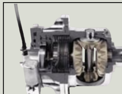
Quadra-Drive II with Electronic Limited-Slip Differentials (ELSDs)
